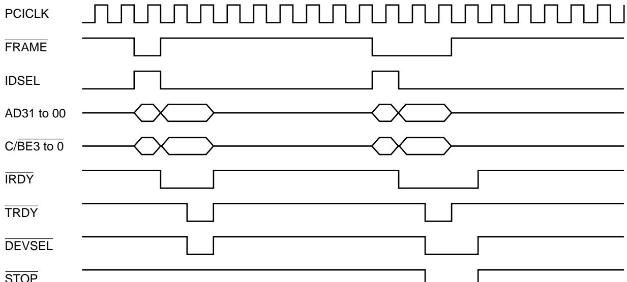
Note: For the access to the configuration register, only one data transfer possible.
