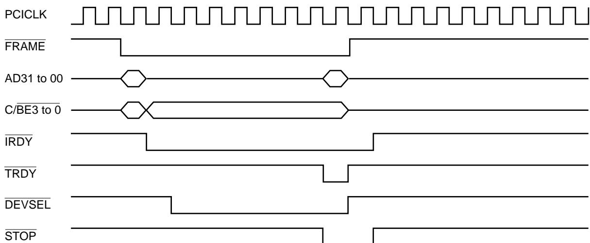
Note: For the read operation of BASIC control registers, only one data transfer possible.
